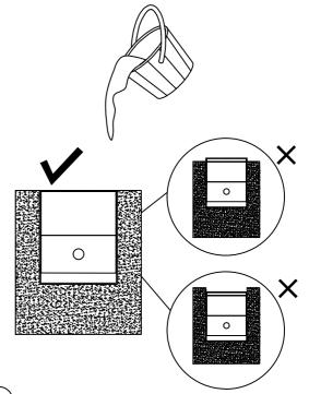
(3) Make Sure the surface of the housing is flushed with the ground
